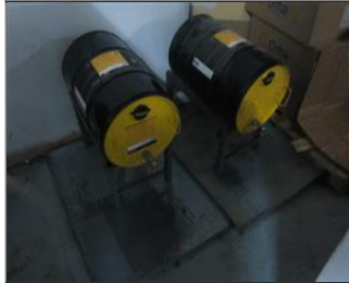
Photo of chemical storage room (if applicable) machine oils with secondary containment.JPG
